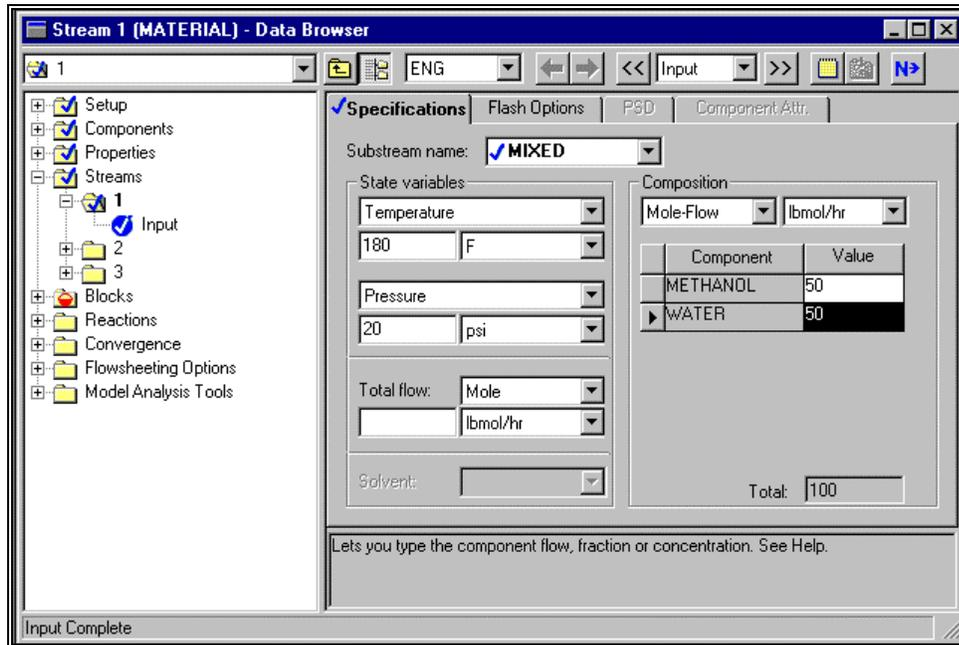
When you enter values in boxes or change default options on Input forms, the specifications you enter and the defaults you modify are shown in black text, and a check mark  will appear next to the sheet name. On the Specifications sheet, the temperature, pressure, and component flow specifications are black, indicating user input.
