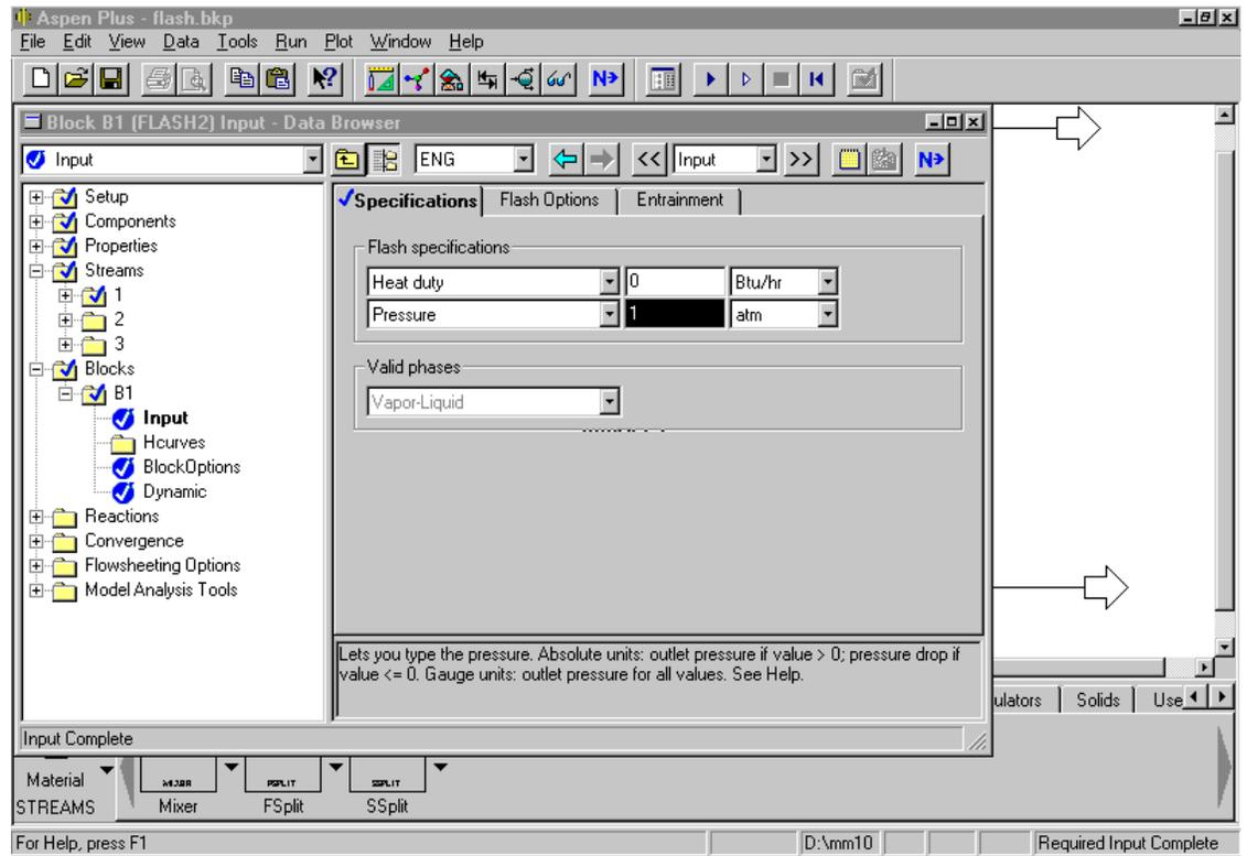
The input for Block B1 is complete as indicated by the check mark on the B1 folder in the menu tree view on the left side of the Data Browser window.
