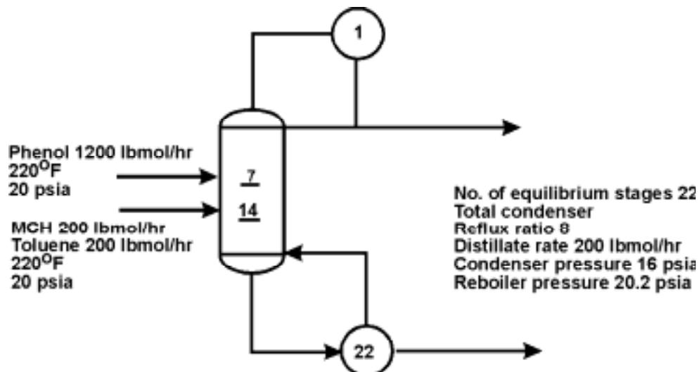
MCH and toluene form a close-boiling system that is difficult to separate by simple binary distillation. In the recovery column in Figure 2.1, phenol is used to extract toluene, allowing relatively pure methylcyclohexane to be recovered in the overhead.
