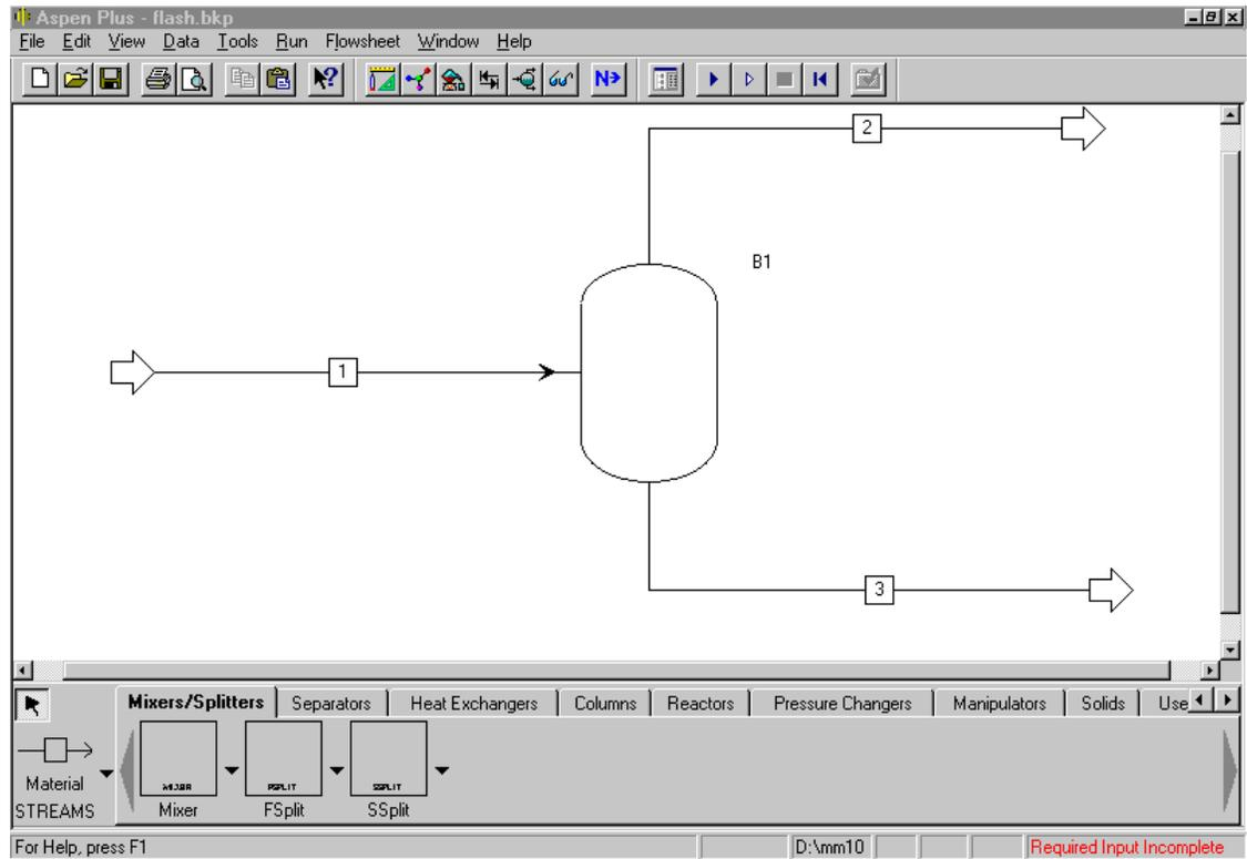
The graphical simulation flowsheet shows the feeds, products, unit operation blocks, and process streams. The Flash simulation has one feed stream (stream 1), two product streams (streams 2 and 3), and one unit operation block (B1).
