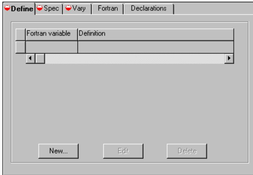
On this Define sheet, you select the simulation variables that you want to sample to calculate the process design specification target. You will identify each sampled variable and give it a unique variable name.
