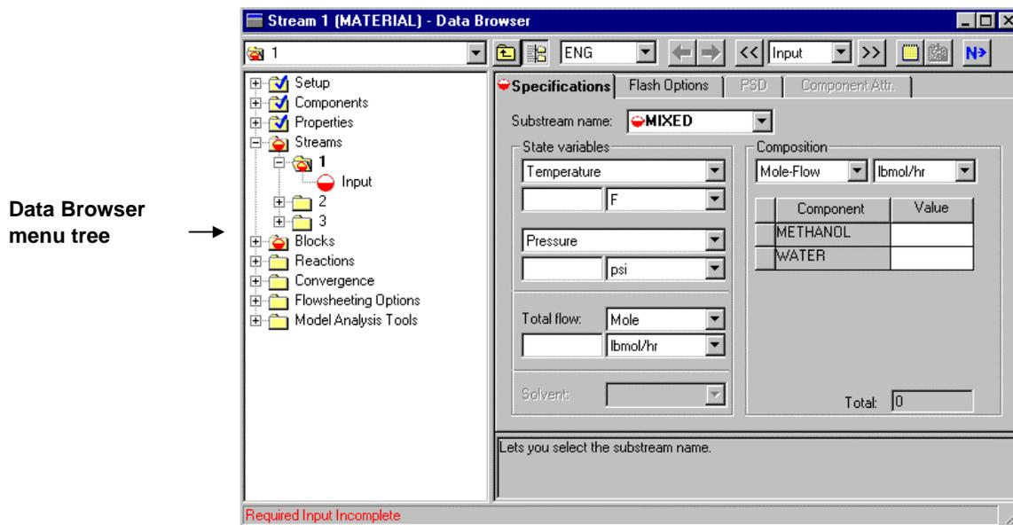
The Data Browser is a sheet and form viewer with a hierarchical menu tree view (on the left side of the window) of the available simulation input, results, and objects that have been defined.
