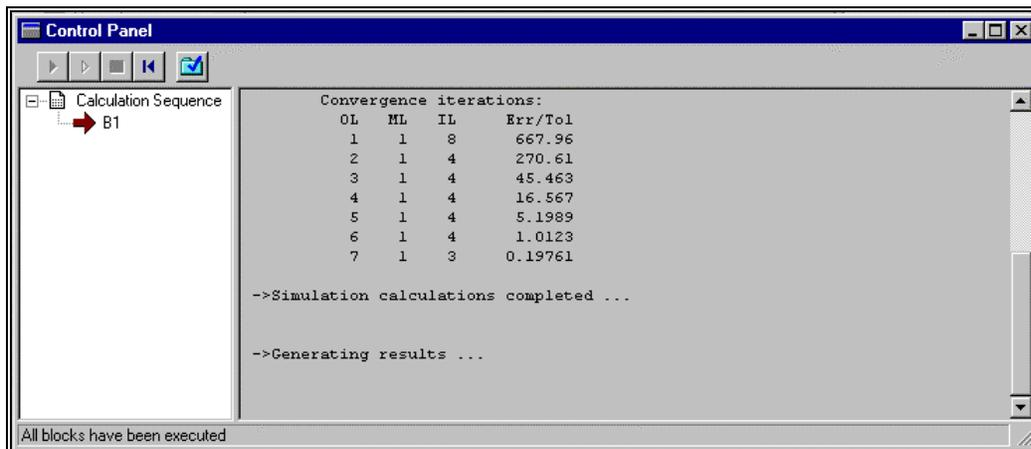
The Control Panel allows you to monitor and interact with the Aspen Plus simulation calculations. For more information on how to control the simulation through the Control Panel, you can either see the *Aspen Plus User Guide*, Volume 1, Chapter 11, or see the topic *Control Panel:about* in the on-line Help.
