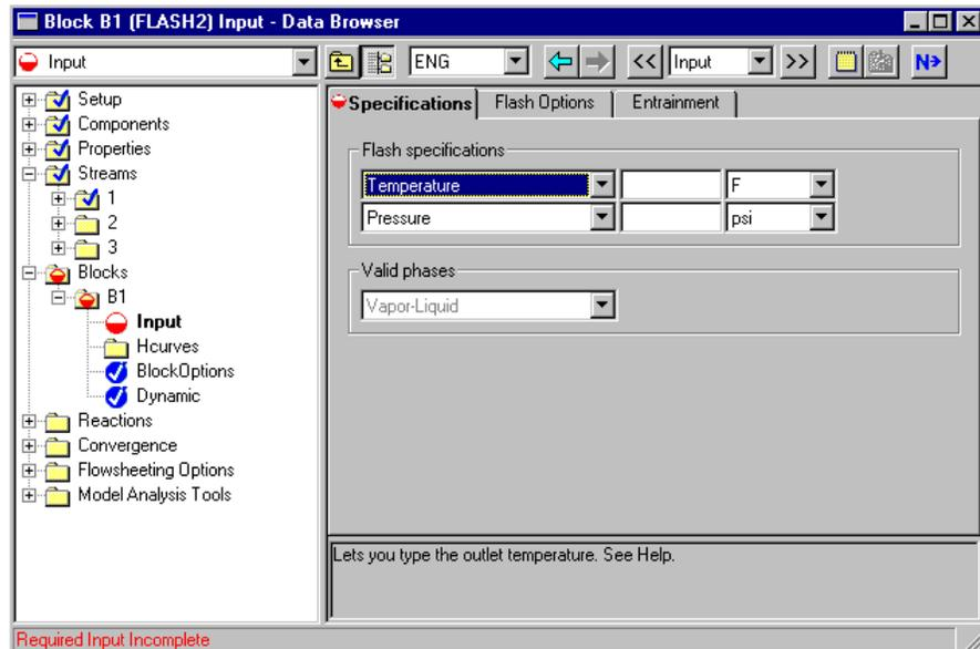
The input data for Block B1 on the Specifications tab is incomplete as indicated by the
