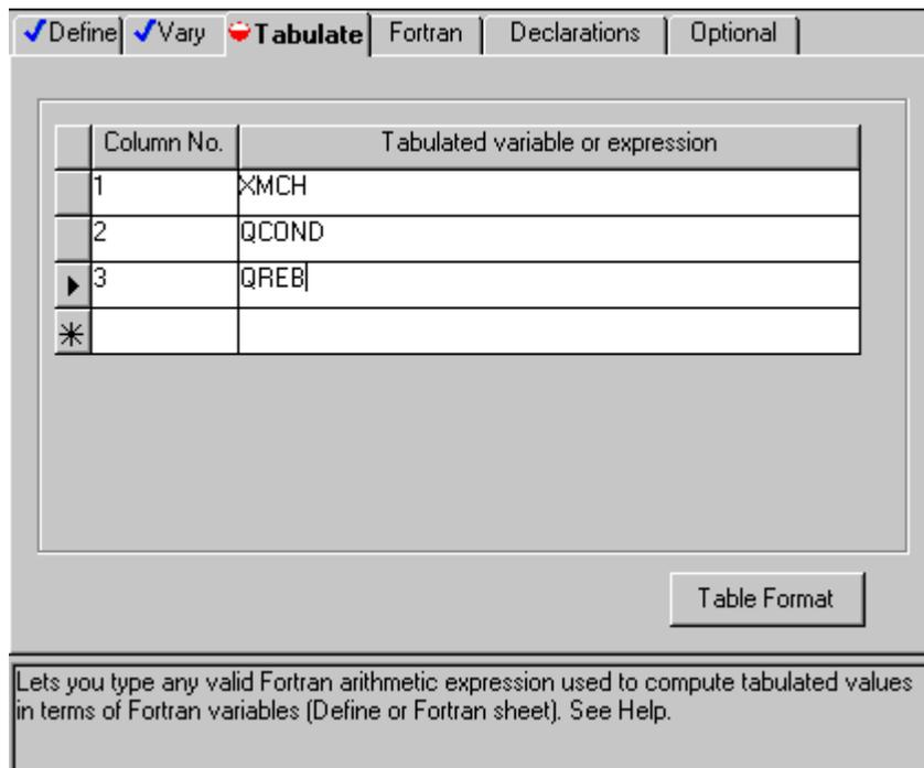
To specify the column labels for condenser duty and reboiler duty:
