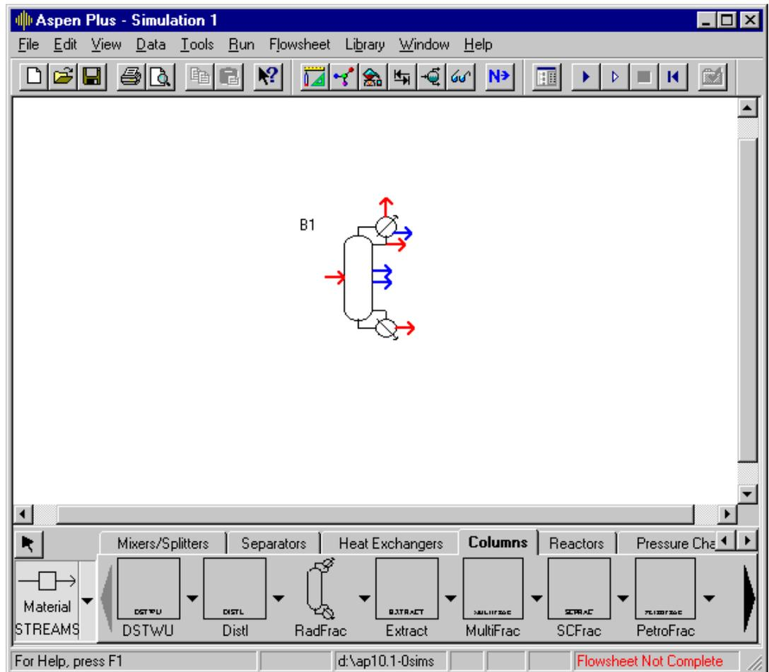
Ports that must have at least one stream connected are shown in red. Optional ports are shown in blue. If you position the mouse pointer over a port for a few seconds, the arrow is highlighted and a description of the port appears.
