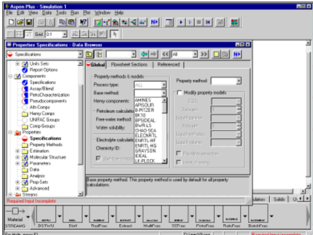
You can get basic information about a base method by using the mouse or the arrow keys to move to the base method and reading the prompt. For more information about a base method, you can move to the base method name and use Help.
