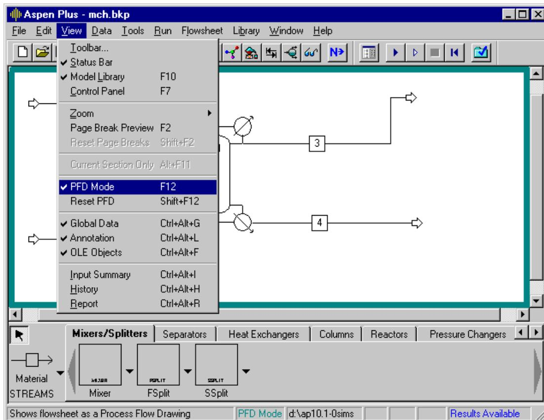
To switch back to Simulation mode, from the View menu, select PFD mode again to clear the check mark. For this example, keep PFD mode on.
