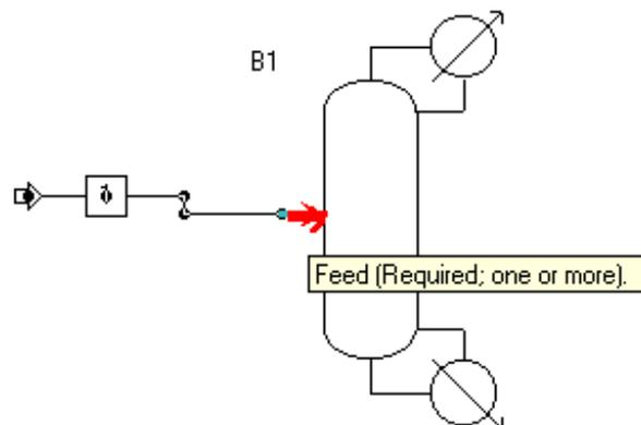
2. Position the mouse pointer where the end of the stream connects to the block.
