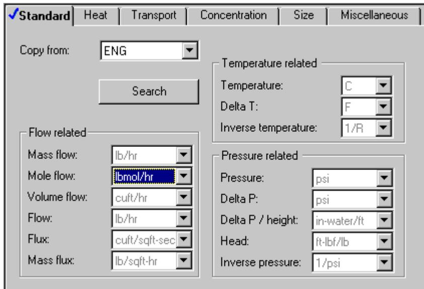
9. On the Temperature box, use the drop down arrow and select C as the temperature.
