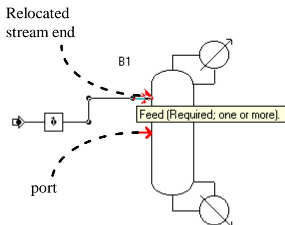
**Tip** You can also move any part of the stream by selecting it and dragging the part of the stream you want to move to its new location.
