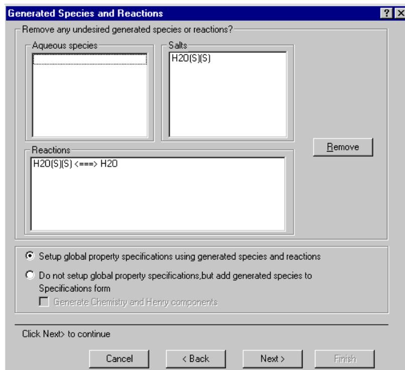
For reactions, arrows pointing in both directions mean ionic equilibrium or salt precipitation. An arrow pointing in one direction means complete dissociation. Generated solid salt components are assigned component IDs with (S) to indicate the solid type.
