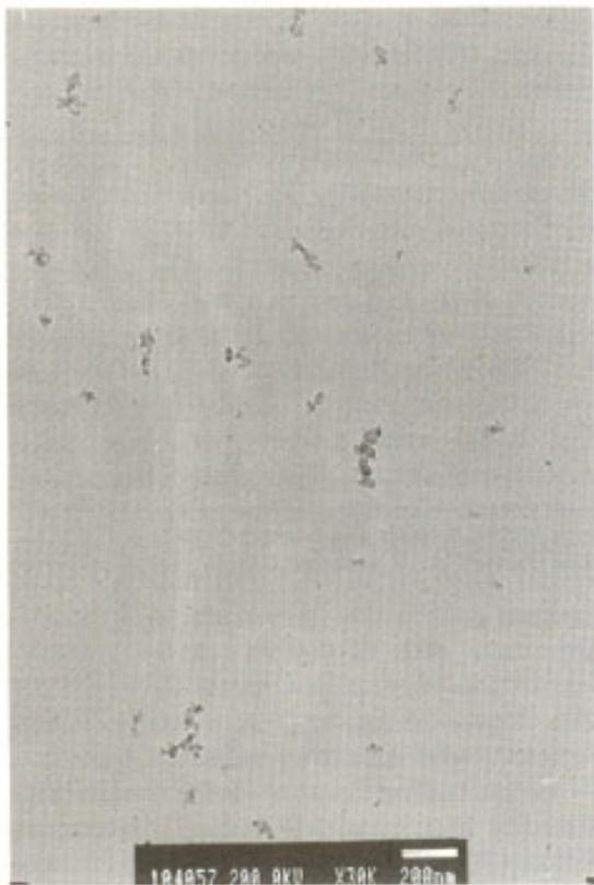
Fig. 1. TEM photograph of soot aggregates along the axis of the weakly-buoyant laminar acetylene/air jet diffusion flame at 0.25 atm. (Flame 1): near the start of soot formation at  $z/d = 2.9$  or a residence time of 4.2 ms. Note, TEM calibration mark is 200 nm long.
