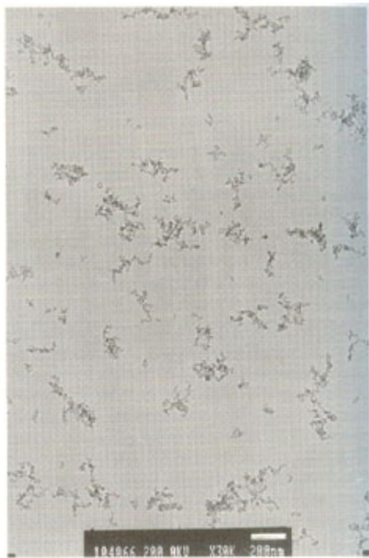
Fig. 2. TEM photograph of soot aggregates along the axis of the weakly-buoyant laminar acetylene/air jet diffusion flame at 0.25 atm. (Flame 1): near the end of the soot formation at  $z/d = 5.7$  or a residence time of 10.8 ms. Note, TEM calibration mark is 200 nm long.
