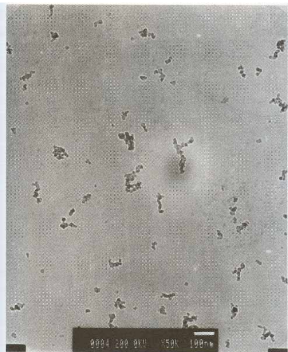
Fig. 2. TEM photograph of soot aggregates along the axis of the C/O = 0.78 flame at z = 22.5 mm.
