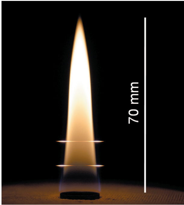
Fig. 2. Color image of the coflowing methane-air laminar jet diffusion flame with horizontal fibers at 11 and 21 mm heights. Exposure settings were 3.3 f , ISO 200, and 8 ms.
