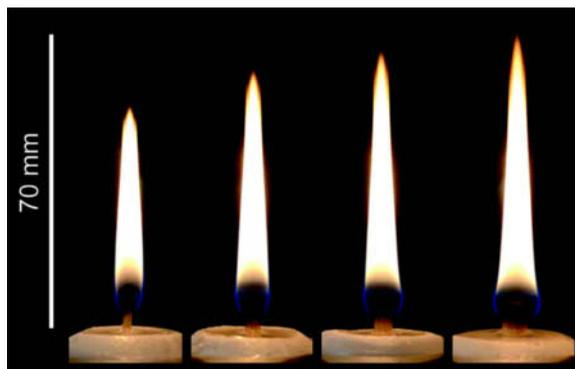
**Figure 1** Color images of tetracosane candle flames at their smoke points. Smoke points are, from left to right, 51.6, 60.0, 65.0, and 67.7 mm. Wick lengths are 10.6, 8.9, 8.2, and 6.6 mm. Wick diameters are 1.9, 3.3, 4.4, and 6.2 mm. These dimensions are slightly different from the mean values for tetracosane reported elsewhere in this paper.
