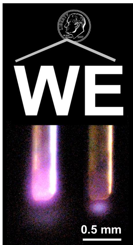
Fig. 1. Images of hydrogen jet flames near their quenching limits in air (left) and in O<sub>2</sub> (right). The word “WE” from a US dime is shown at the same scale as the flames.
