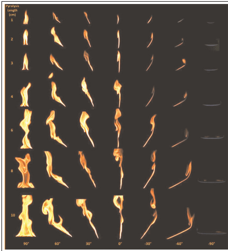
Figure 2. Methanol flame shapes at various orientations and plate (pyrolysis) lengths.
