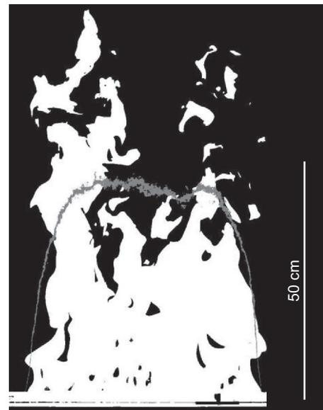
Fig. 2. Sample image depicting flame height image processing technique. A single flame snapshot (black/white regions) is overlaid with the corresponding mean flame shape (gray contour).  $X_{O_2}=0.20$ ,  $L_f=45$  cm.
