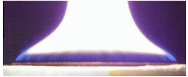
Fig. 8. Ethylene flame on the BRE 50 mm burner.
